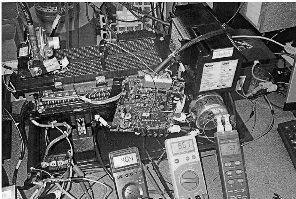
Fig. 2. Nexa™ power module and experimental hardwares. Stack #768 voltage at 40.4 V and the 27th MEA's voltage at 0.861 V with no external load at room temperature.
